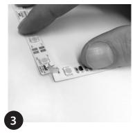
With the bend tabs in place. Mock up the installation by making the required bends on the UNI FX where required. Once product is bent to the rough installation shape, stick down 1 section of 3M backing at a time to ensure good fixation.
