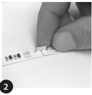
Prepare sections of UNI FX for bending where required. First bend the bend tab vertically upwards.
