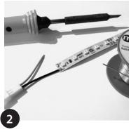
Carefully solder prepared cable to marked solder pads. Minimise contact time to avoid excessive heating of the strip.
